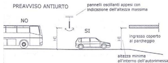
Figure 11. Technical device placed before the garage, to avoid damage to tall vehicles
