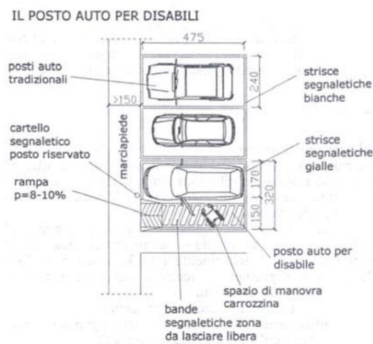
Figure 9. Minimum dimensions of a parking space for users with mobility difficulties
